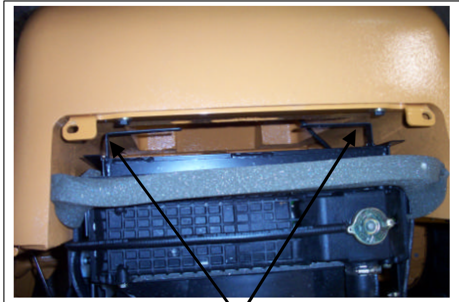
Top condenser mount brackets bolted in place into existing threaded holes on the oil cooler flanges.
