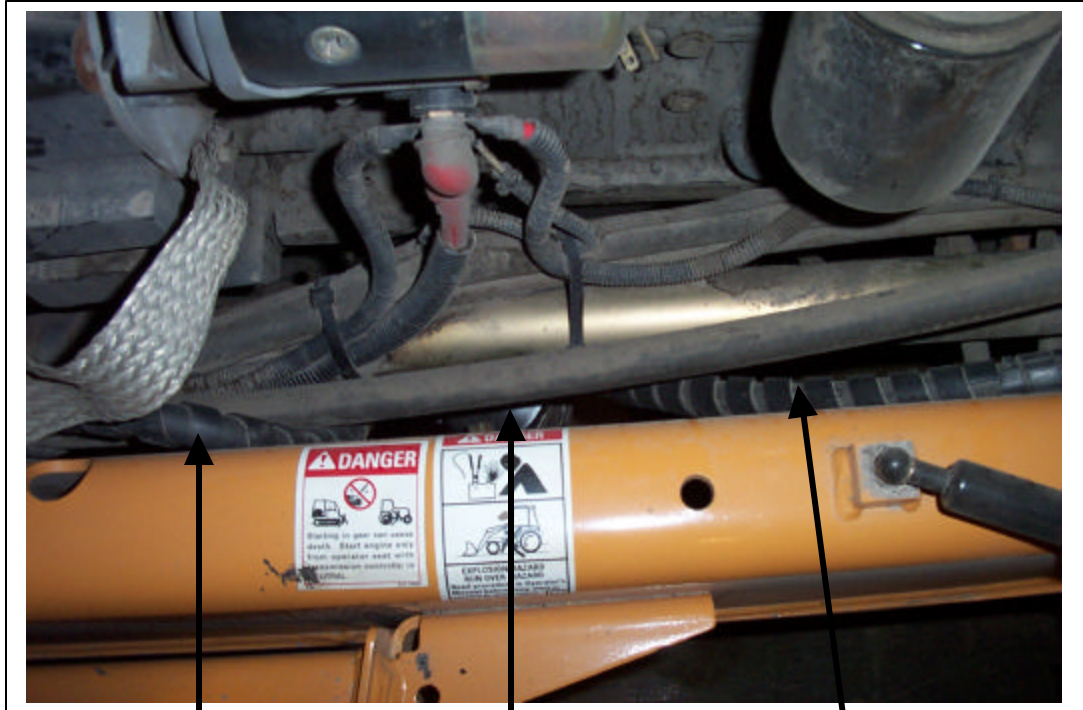
5/16" hose from the drier outlet to the evaporator box in the cab.
