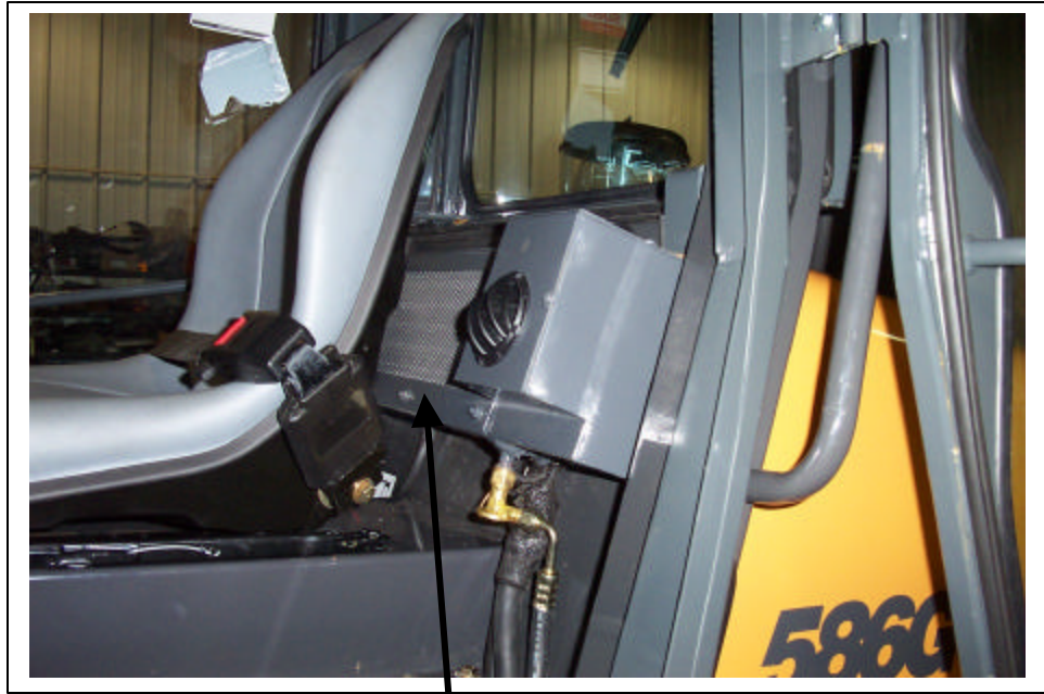
Evaporator box mounted to the engine firewall just below the skinkit cab enclosure.
